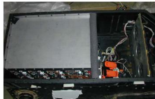
Figure 4. XM1124 First generation hybrid pack.
